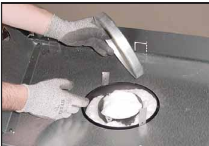
Figure 9.3 Remove the seal cap.
